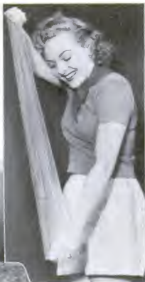
This elastic plastic core for safety glass enables a shattered pane to be rolled up like a carpet, at left
